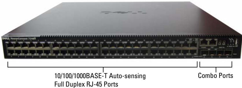
Figure 1-6. PowerConnect 7048R with 48 10/100/1000BASE-T Ports
